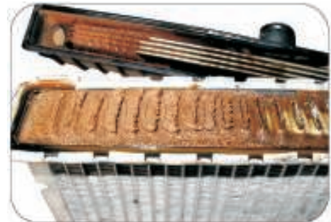
Large deposit of foreign matter inside the radiator tank
