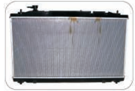
Leak caused by contaminated coolant
