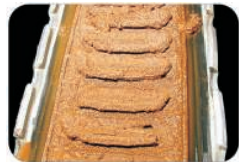
Large deposit of foreign matter inside the radiator tank
