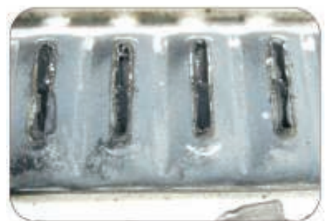
The tubes on the header plate have become brittle and broken away
