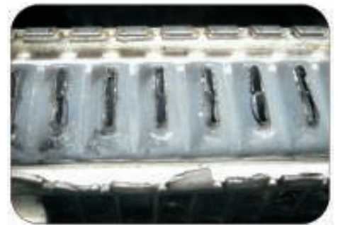
Blackening of the header plates. The tubes and brazed joints have corroded away.
