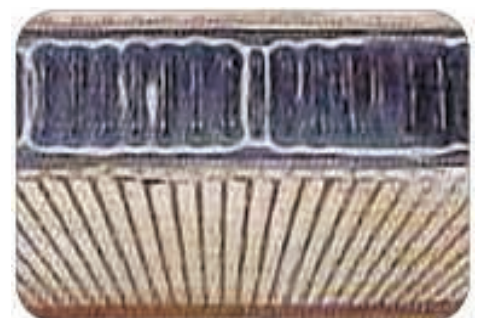
Top header plate discoloured
