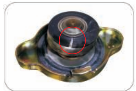
Cracked / worn gasket
