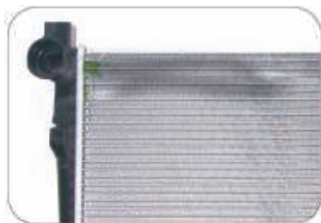
Coolant leakage, as a result of thermal shock.
